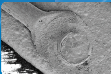
SEM images showing preserved copper wires
